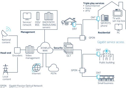
GPON Gigabit Passive Optical Networ OLT Optical Line Terminal ONT Optical Network Terminal
